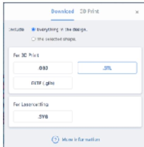
Load the STL into your 3D printing software and slice the model for 3D printing. You can slice and print it in the lowest resolution. Once printed, you can use either the textured top side of the stamp or the smoother surface that was in contact with the print bed. These will give different effects to your final tile.
